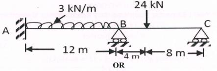
6 Analyze the continuous beam as shown in figure below by slope deflection method. Support B sinks by 10 mm. Take E = 200 GPa and  $I = 16 \times 107$  mm4. Draw the bending moment diagram
